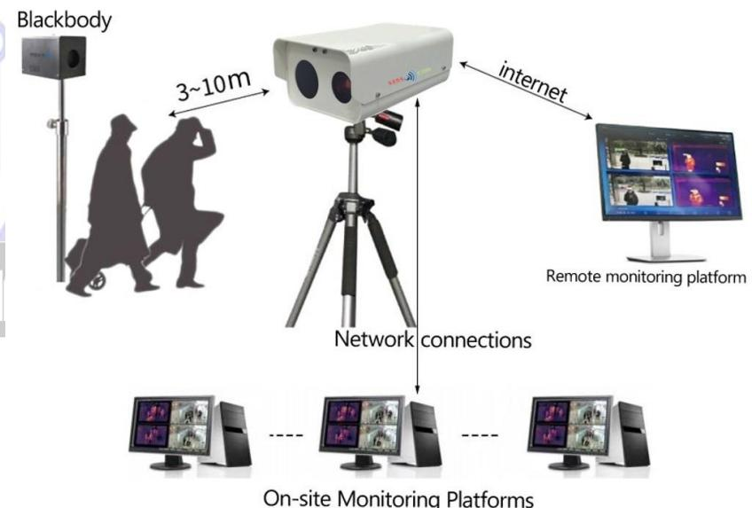
The field of view of the visible light camera can be adjusted to the infrared thermal imager. Each infrared and visible camera can output two video signals at the same time, and connect to the computer using the network port.
